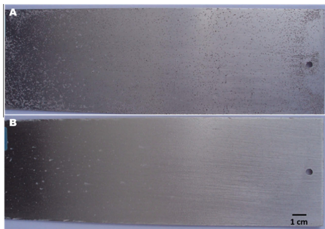
Fig. 8. Coated AA2024 with (A) unmodified sol-gel and (B) with sol-gel containing MBT@PU-MC, after 168 h in NSS.
