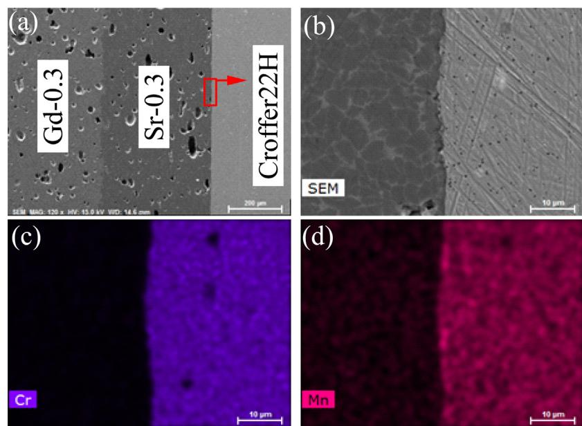
Fig. 5. SEM image and elemental mappings at the Interface between Gd-0.3 GC/Sr-0.3 GC/Crofer22H after heat treating at 850 °C for 100 h.
