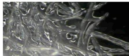
**Figure 2.** Optic microscope image of UHP-treated (400 MPa, 20 min) and xylanase hydrolyzed cellulosic fibres of *E. globulus* bleached kraft pulp.
