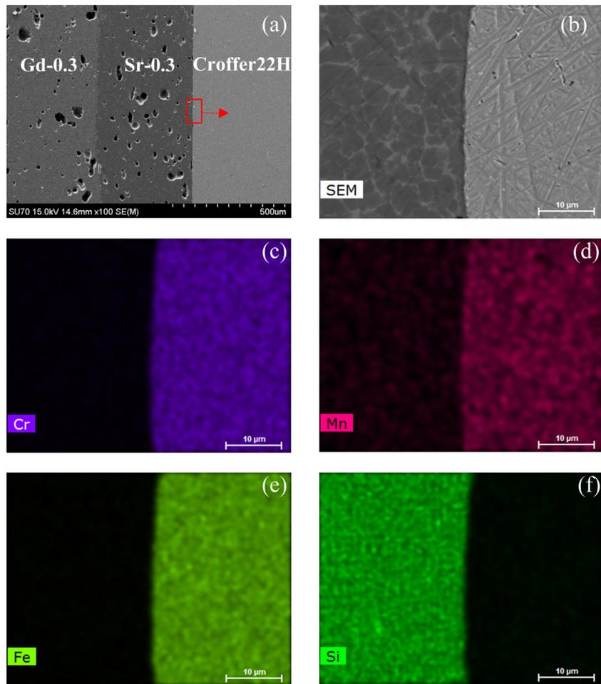
Fig. 4. SEM image and elemental mappings at the interfaces between Gd-0.3 GC/Sr-0.3 GC/Crofer22H after heat treatment at 850 °C for 1 h.
