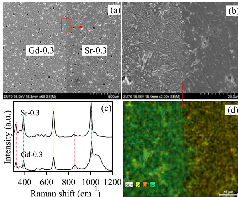
Fig. 2. Interface between Gd-0.3 and Sr-0.3 glass-ceramics after heat treating at 850 °C for 100 h: (a) and (b) SEM images; (c) Raman spectra; (d) elemental mapping.
