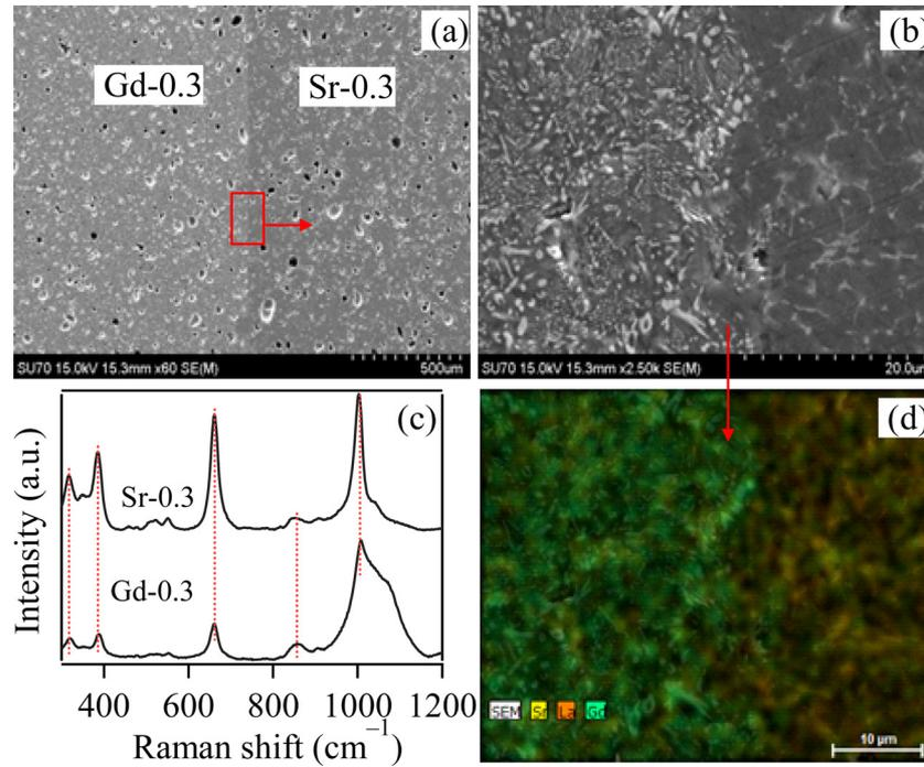
Fig. 1. Interface between Gd-0.3 and Sr-0.3 glass-ceramics after heat treating at 850 °C for 1 h: (a) and (b) SEM images; (c) Raman spectra; (d) elemental mapping.
