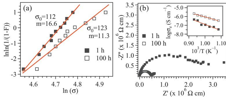
Fig. 3. (a) Weibull distributions of flexural strength values for the Gd-0.3/Sr-0.3 bi-layered glass-ceramics heat treated at 850 °C for 1 h, and (b) impedance spectra obtained at 800 °C in air of bi-layered glass-ceramics. The inset in (b) shows the temperature dependence of the electrical conductivity.
