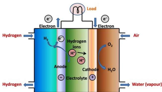
FIGURE 11.7 Schematic representation of a solid oxide fuel cell. Reproduced with permission from A.M. Abdalla, S. Hossain, A.T. Azad, P.M.I. Petra, F. Begum, S.G. Eriksson, et al., Nanomaterials for solid oxide fuel cells: a review, Renew Sust Energ Rev 82, 2018, 353–368.
