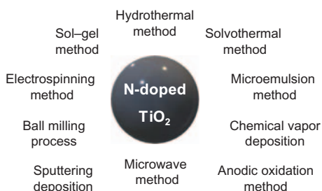
FIGURE 21.21 Schematic diagram illustrating the different synthetic routes for the preparation of N-doped TiO 2 .
