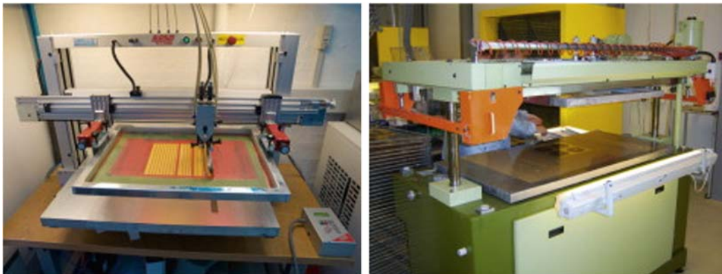
FIGURE 21.9 Examples of laboratorial (left) and industrial (right) screen-printing apparatus. Reproduced from Krebs FC. Fabrication and processing of polymer solar cells: a review of printing and coating techniques. Sol Energy Mater Sol Cell 2009;93:394–412 [27] with permission from Elsevier.
