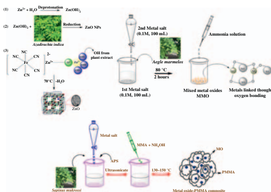
FIGURE 13.9 Various green strategy for the synthesis of doped metal hexacyanoferrates, bimetallic oxides simple, and doped with PMMA.
