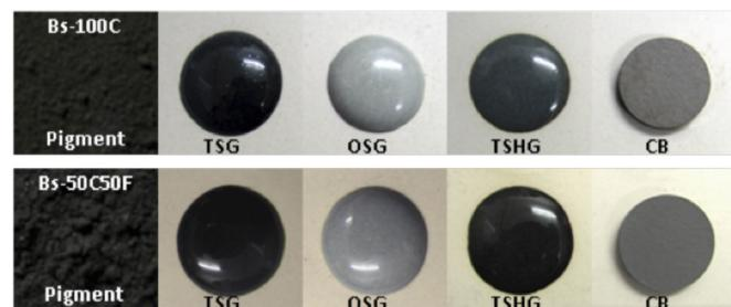
**Figure 1:** Ceramic pigments prototypes. Colors developed by the pure pigments (left), by the glazes - transparent and opaque (centre) containing 5 wt% pigment, and by ceramic bodies containing 10 wt % pigments (right). Protótipos de pigmentos cerâmicos. Cores desenvolvidas pelos pigmentos puros (esquerda), pelos esmaltes - transparente e opaco (centro) contendo 5 wt%, e pelos corpos cerâmicos contendo 10 wt% (direita).
