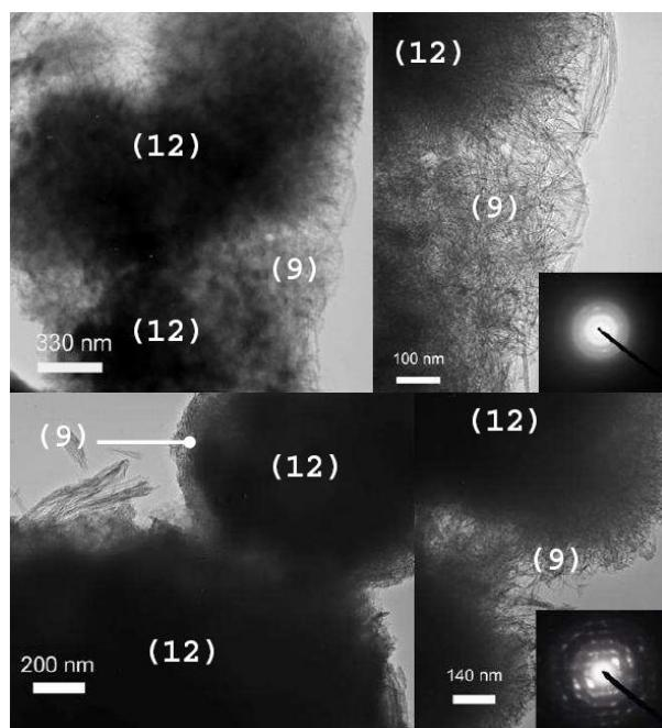
**Figure 1:** TEM micrographs of SrAl<sub>2</sub>O<sub>4</sub>: Ce<sup>3+</sup>, Dy<sup>3+</sup>, Eu<sup>2+</sup> (12), encapsulated with a semi-crystalline TiO<sub>2</sub> layer (9). Micrografias de TEM de SrAl<sub>2</sub>O<sub>4</sub>: Ce<sup>3+</sup>, Dy<sup>3+</sup>, Eu<sup>2+</sup> (12), encapsulados com uma camada de TiO<sub>2</sub> semi-cristalino (9).
