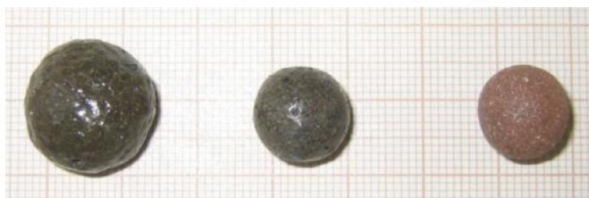
**Figure 1:** Lightweight aggregate prototypes. Protótipos de agregado leve.
