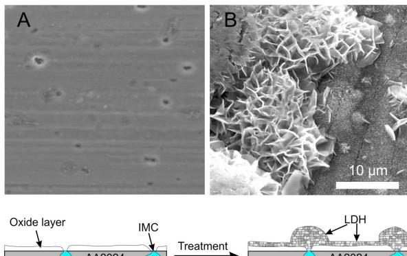
**Figure 1:** SEM images of the substrate (A) and the substrate coated with Zn-Al LDHs intercalated with V<sub>2</sub>O<sub>7</sub><sup>4-</sup>(B). Imagens de SEM do substrato (A) e do substrato revestido com HDLs de Zn-Al intercalados com V<sub>2</sub>O<sub>7</sub><sup>4-</sup>(B).
