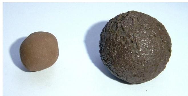
**Figure 1:** View of unfired (left) and fired (right) samples.
