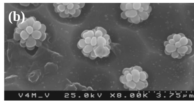
**Figure 1&2:** Microstructure by scanning electron microscopy of the present invented glass after annealing (a) 3000x and (b) 8000x. Microestrutura por microscopia electrónica de varriamento (a) 3000x e (b) 8000x do vidro inventado após recocimento.
