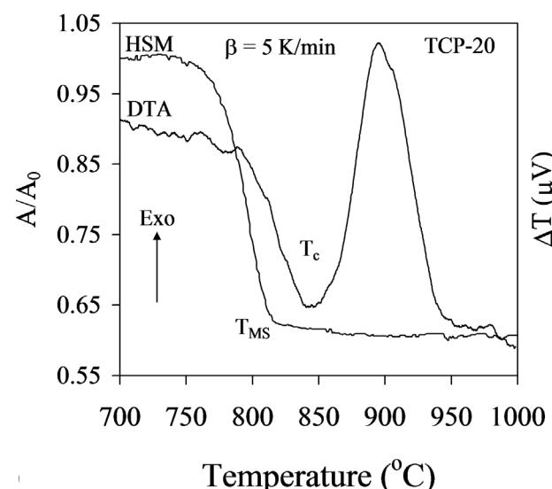
**Figure 1:** Comparison between hot-stage microscopy (HSM) and differential thermal analysis (DTA) curves for the glass TCP-20. Heating rate: 5 K/min. Comparação entre as curvas de microscopia de aquecimento (HSM) e de análise térmica diferencial (DTA) para o vidro TCP-20. Taxa de aquecimento: 5 K/min.
