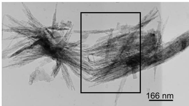
**Figure 1:** Example of aligned luminescent aluminate  $\text{SrAl}_2\text{O}_4:\text{Ce}^{3+}, \text{Eu}^{2+}, \text{Dy}^{3+}$  nanowires. Exemplo de nanofios de alumínato luminescente alinhado  $\text{SrAl}_2\text{O}_4:\text{Ce}^{3+}, \text{Eu}^{2+}, \text{Dy}^{3+}$ .
